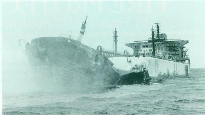
The fire is extinguished on the NASSIA with the majority of the crude oil tanks left intact. Some tanker fires can take weeks to finally extinguish. In most instances, it takes days to simply cool a vessel before a foam attack can be undertaken. This operation took only three days before completion. [© PIM KORVER FILM + VIDEO]
