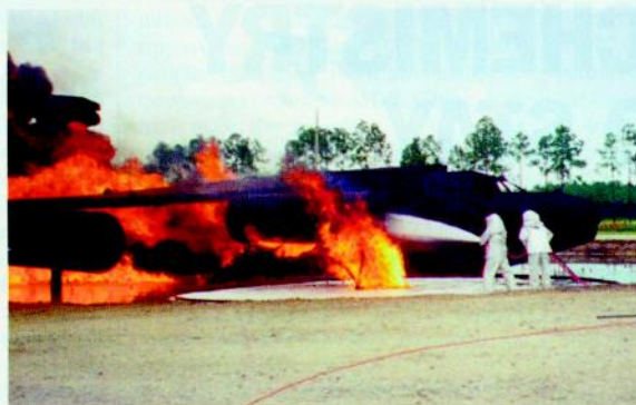
Pyrocool FEF being used to extinguish a pressurized, obstructed, multilevel military jet fuel engine fire at Tyndall Air Force Base in Florida. Test duplicates an actual crash at Travis AFB in California that took hours to extinguish. The test fire was extinguished in 34 seconds.
